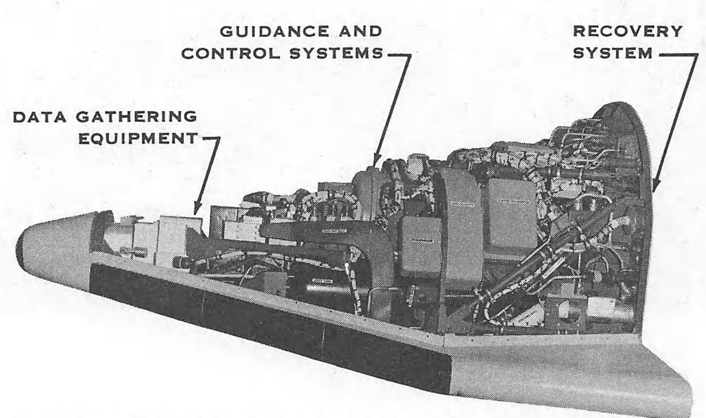
AEROTHERMODYNAMIC STRUCTURAL MOCK-UP
