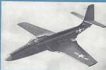
Night fighter, the F2H-2N Banshee, with radar nose
