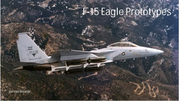
The second twin-seat prototype, 71-0291, is probably the best-known of the Eagle prototypes. Following the test program at Edwards AFB, the aircraft was used by McDonnell Douglas as their dedicated test and development machine. It is seen here on 10 February 1976, carrying a load of Sparrow missiles and bombs. (all photos Mark Nankivil, Greater St Louis Air and Space Museum, unless credited otherwise)
