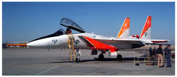
F-15A-4-MC - 71-0287 made its first Flight on 25 August 1973; it was used as the test aircraft for spin recovery and angle of attack trials and fuel systems tests. For spin recovery purposes, the aircraft had a small box-like structure attached to the rear fuselage which housed the anti-spin recovery parachute; this can be seen on this photograph, taken at Edwards on 25 November 1975 (Thomas Brewer via Stephen Miller).
