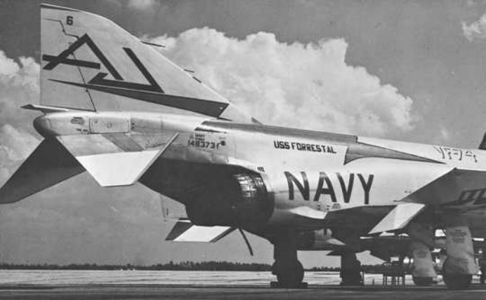
Twin engines capable of 34,000-lbs total thrust power Phantom II to Mach 2.5 speeds. Down-swept tail aids controllability through full speed range.
